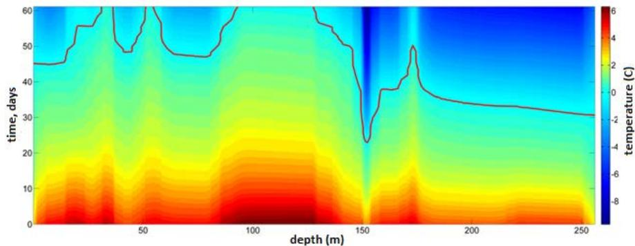
Fig. 3. Numerical results of temperature evolution in control boreholes.
