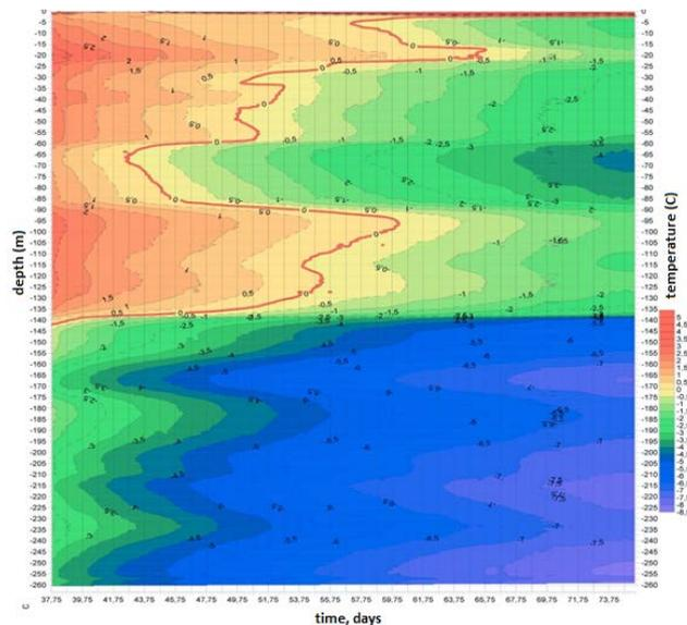
Fig. 2. Temperature evolution in control boreholes.
