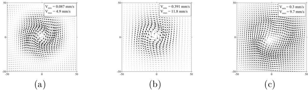
Figure 4: Mean vector velocity fields at  $z = 15\text{ mm}$ , heat power  $P = 17\text{ Wt}$ ,  $\Omega = 0.081\text{s}^{-1}$ : a - PMS-10, b - PMS-5, c - PMS-3
