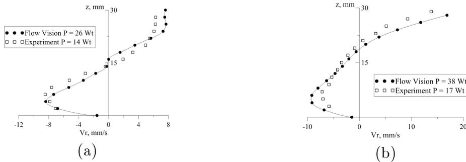
Figure 6: Mean radial velocity profiles (PMS-3): a -  $P = 14 \text{ Wt}$ ,  $\Omega = 0.081 \text{ s}^{-1}$ , b -  $P = 17 \text{ Wt}$ ,  $\Omega = 0.041 \text{ s}^{-1}$
