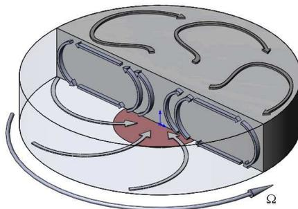
Figure 2: The structure of main flow in a rotating frame
