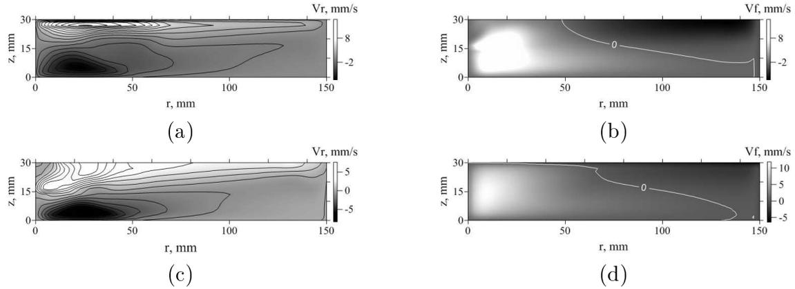
Figure 5: Mean radial (a, c) and azimuthal (b, d) velocity fields obtained from Flow Vision (PMS-3): a, b -  $P = 26 \text{ Wt}$ ,  $\Omega = 0.081 \text{ s}^{-1}$ , c, d -  $P = 38 \text{ Wt}$ ,  $\Omega = 0.041 \text{ s}^{-1}$
