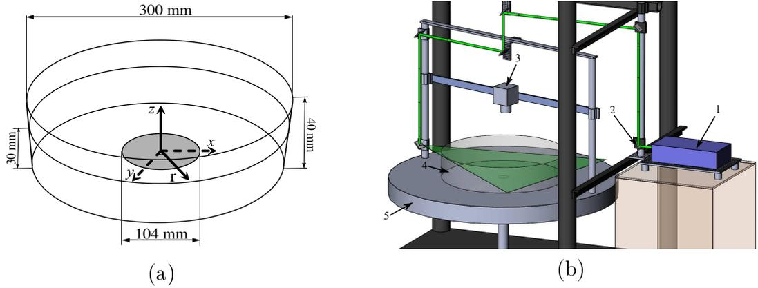
Figure 1: Experimental setup: (a) Dimensions and location of the coordinate system, (b) - Measurement system
