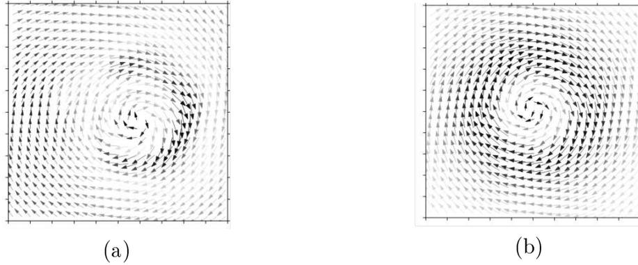
Figure 7: Instantaneous - a and mean - b vector velocity field at  $z = 15$  mm,  $P = 14$  Wt,  $\Omega = 0.081s^{-1}$ , PMS-3
