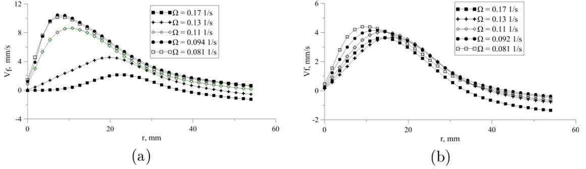
Figure 3: Mean azimuthal velocity profiles for height  $z = 15\text{mm}$  for regimes with different rotation rates and fixed heat power  $P = 17\text{wt}$ : a - PMS-5, b - PMS-10
